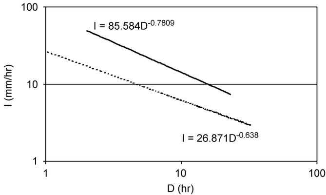
Fig. 2. Rainfall duration/intensity relationship for triggering shallow landslides in the southern Apuan Alps. A lower and an upper threshold curves are recognizable (after Giannecchini, 2006, modified).
