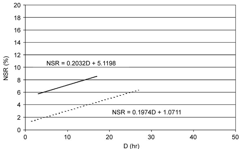
Fig. 4. Rainfall duration/NSR relationship for triggering shallow landslides in the southern Apuan Alps. A lower and an upper threshold curves are recognizable (after Giannecchini, 2006, modified).
