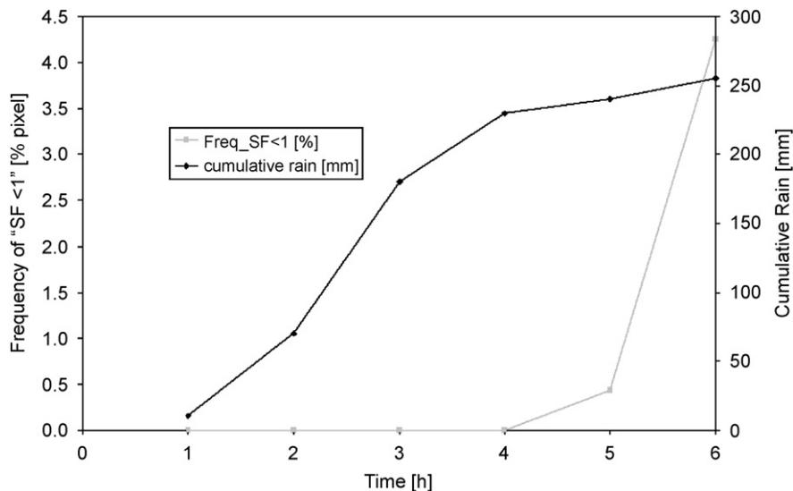
Fig. 6. Number of unstable cells and cumulative rainfall for the first 6 h of the simulation.
