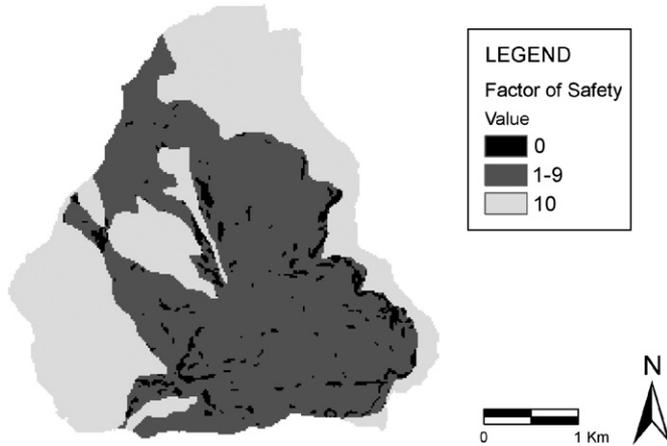
Fig. 5. Landslides activity reported in terms of unstable cells (factor of safety < 1) after the first 6 h of the simulation.
