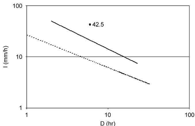
Fig. 7. Mean precipitation per hour (for the first 6 h) plotted in the graph. Rainfall intensity/NSR for triggering shallow landslides in the southern Apuan Alps.
