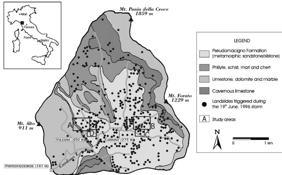
Fig. 1. Lithologic sketch map of the Cardoso Torrent basin and location of the main landslides triggered by the June 19, 1996 rainstorm (after D'Amato Avanzi et al., 2004, modified).
