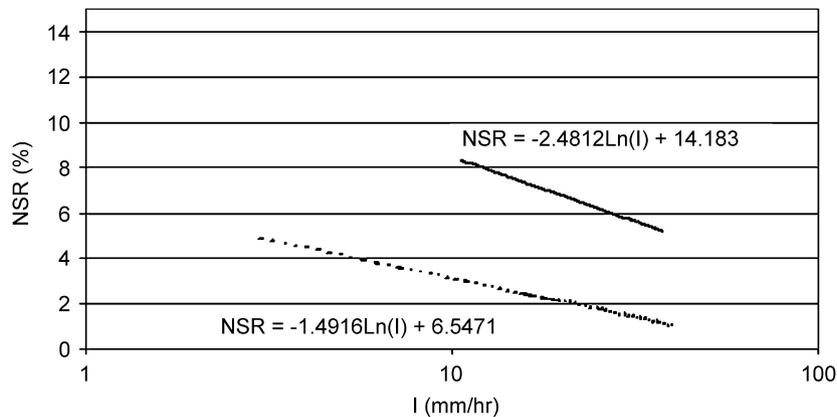
Fig. 3. Rainfall intensity/NSR relationship for triggering shallow landslides in the southern Apuan Alps. A lower and an upper threshold curves are recognizable (after Giannecchini, 2006, modified).
